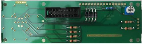
Inspect carefully the assembly and soldering. Once the LCD is mounted (next step), it becomes quite difficult to rework any soldering or assembly of the bottom-side!
