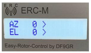
Adjust the contrast with the potentiometer R1 on the backside of the HID-PCB.
