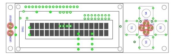
**Hint:** Only solder 1 leg of the switches and LEDs, check for alignment and than solder the remaining pins.
