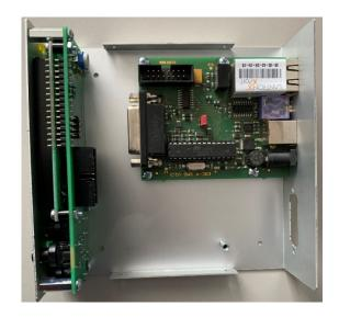
Fold the 15-pole flat-ribbon-cable as shown and put the DSUB-connectors as shown and mount the female-DSUB-connector to the back-panel of the housing with the 2 UNC4 5mm distance-bolts.
