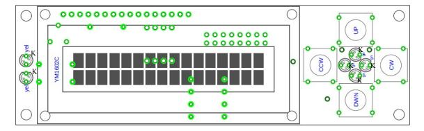
Put the 19mm domes on top of the switches.
