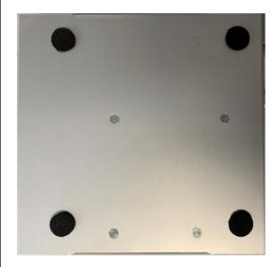
Remove the protection-foil from the LCD and mount the HID into the desktop-housing with 4 countersunkscrews M3x4.
