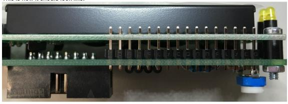
Mount the 4 distance-bolts M3x15 with 4 screws M3x6 on the PCB.
